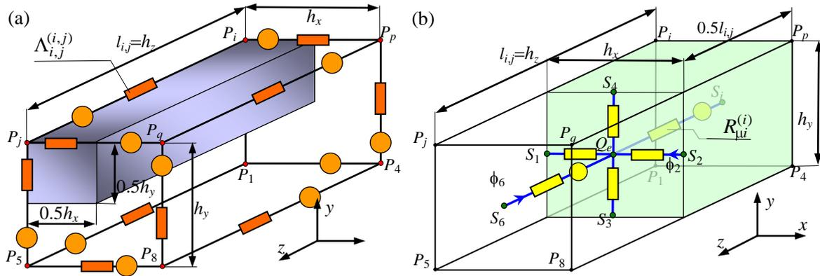
Fig. 3. Geometric forms representing permeance (a) and reluctance (b).
