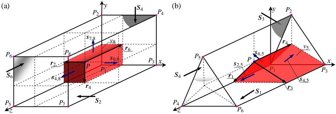
Fig.1. Geometric representation of interpolation functions of hexahedron (a) and 9-edge pentahedron (b).
