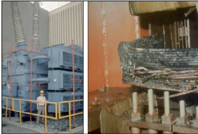
Generator step-up transformer damaged by March 1989 solar storm.
