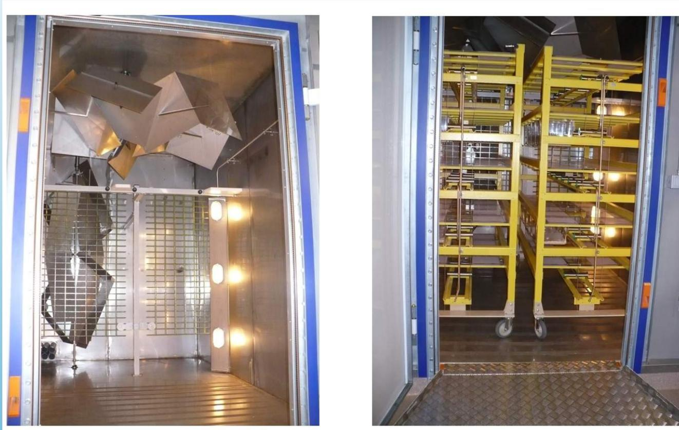
**A room shielded from penetrating EMFs containing an excitation antennae and ventilation panels. Field exposures emanate from multiple angles (all directions), while rotating paddles distribute the fields to create a statistically homogeneous electromagnetic environment. No limit on daily exposure time, no comparable historical control.**
